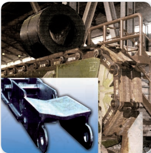
Coil carrying chain pitch 630 mm. - for coils till dia. 1650 mm - for coils till 40000 kg - for coils till 600 °C
