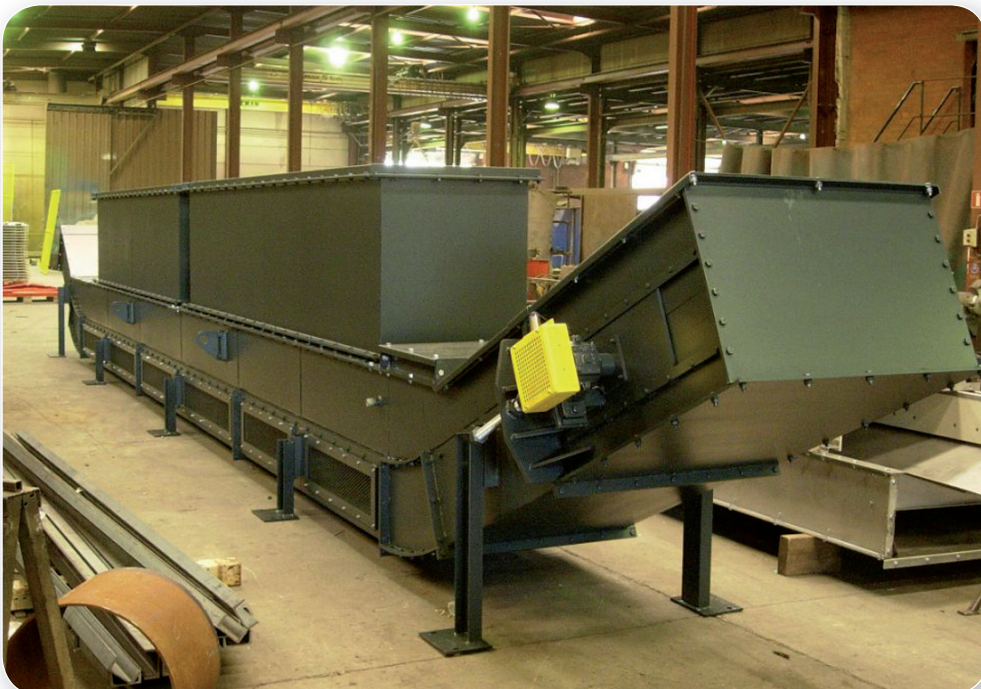
Scraper conveyor casing for extraction under bunker or hopper.
