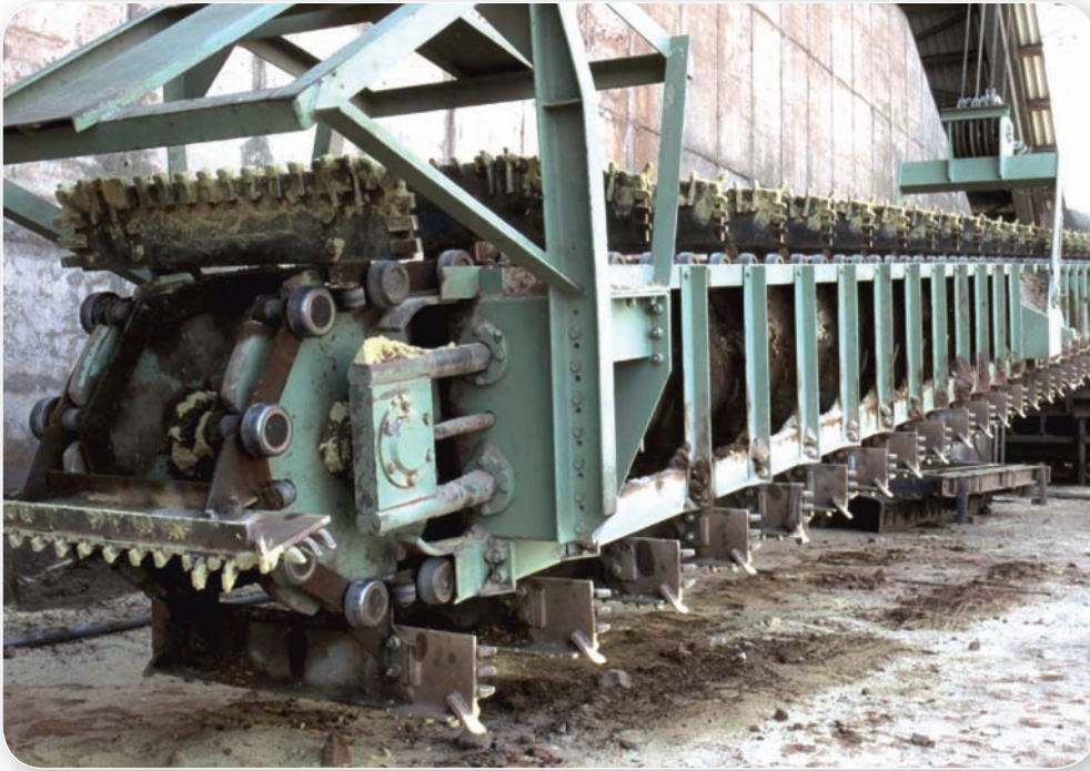
Scraper chain pitch 250 mm for cement Industry
